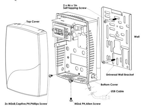
Figure 3. Mounting the HUSB onto the Universal Wall Bracket
